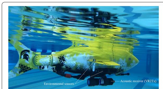
**Fig. 1** Gliding robotic fish. The modified version of GRACE with bottom-mounted telemetry receiver
